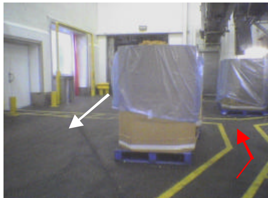
Figure 13: Illustration of how the pallet creates a blind corner if pedestrians are approaching from the direction of the red arrow and forklift trucks moving in the direction of the white arrow. On the basis of this observation, a recommendation was made at the case study organisation to create (and demark) specific areas for the storage of pallets and to remind forklift truck drivers of the danger of placing pallets (obstructions) at the end of aisles and at intersections. Finally, it
