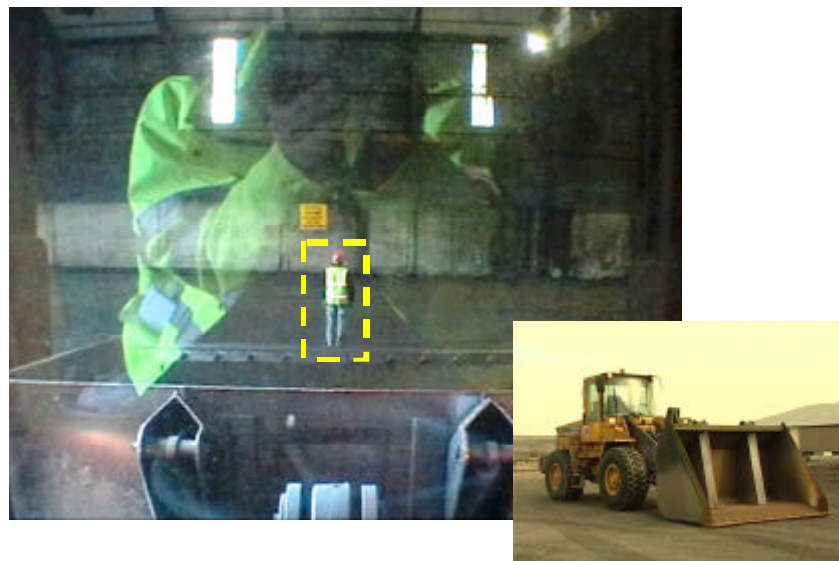
Figure 4.0: view from the cab of a Shovel-Loader showing veiling effect caused by light reflecting off the driver’s high-visibility jacket.
