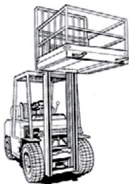
Figure 1 Counterbalance truck with non-integrated working platform
