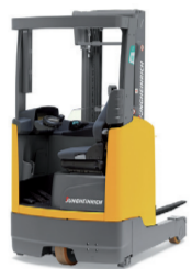
D1 | Rider | Electric Reach & straddle trucks 3-8m lift
