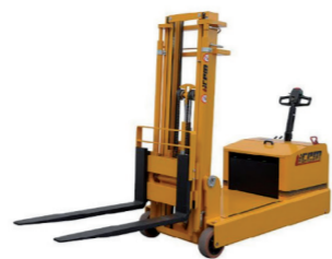
A3 | Pedestrian | Electric Counterbalance lift trucks
