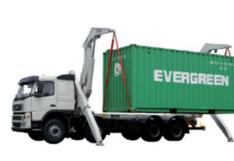
G3 | Rider | I.C.E. Side loader container handling trucks
