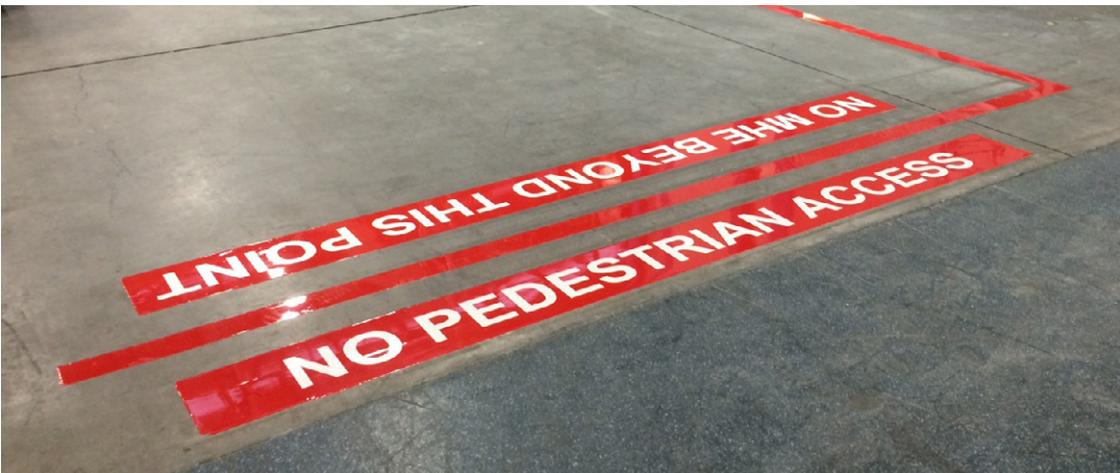
**Loading and Unloading Zones** – these should be segregated from parking areas and where necessary, a segregated pedestrian safe zone should be created.
