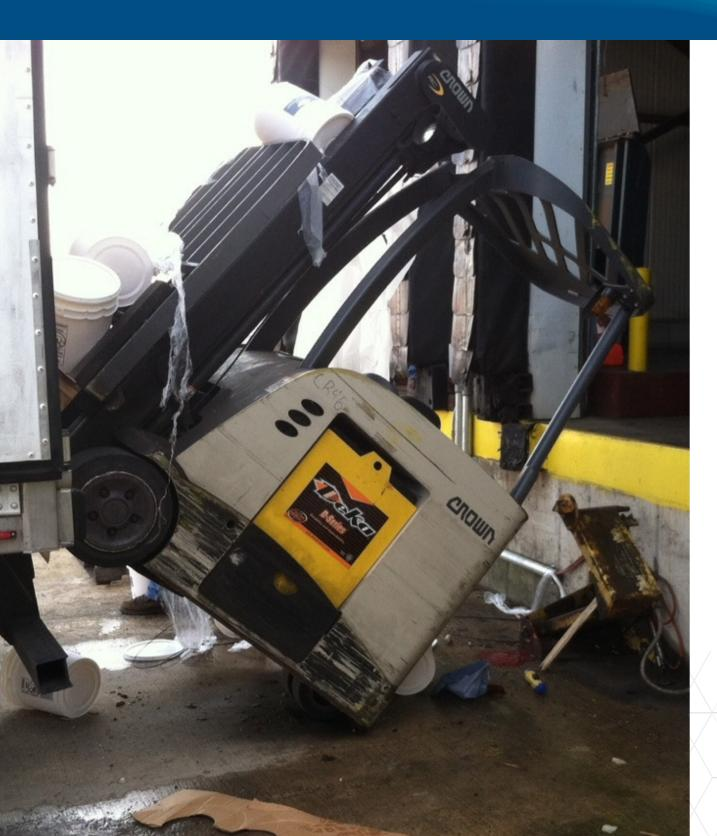
The i-Stop system is designed precisely to prevent recurrence of accidents at logistic centers. **The truck** driver who park at the platform will not be able to start unloading or loading goods before securing the truck's tires with Solan's unique wireless stop-breaker: the i-Stop. Only when i-Stop is attached to the truck wheels it become possible to open the logistics center's platform door and the truck can no longer move from its place. Now the forklift driver can perform his duties safely.
